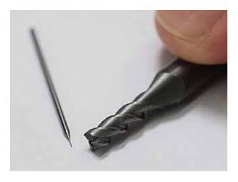
Low-stress aluminium (closeup with micro tool). Machining tool with 0.15 mm diameter.
